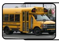
A <u>Type "A"</u> school bus is a van conversion or bus constructed utilizing a cutaway front-section vehicle with a left side driver's door. The entrance door is behind the front wheels. The definition includes two classifications:
